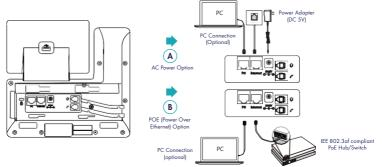
**Note:** The IP phone should be used with Yealink original power adapter (5V/1.2A) only. The use of the third-party power adapter may cause damage to the phone. If you are connecting a PC to your phone, we recommend that you use the Ethernet cable provided by Yealink. If inline power (PoE) is provided, you don't need to connect the power adapter. Make sure the hub/switch is PoE-compliant.
